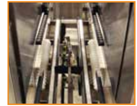
HIGH SPEED ROTARY UPSTACKER WITH SURGE/METERING BELTS
